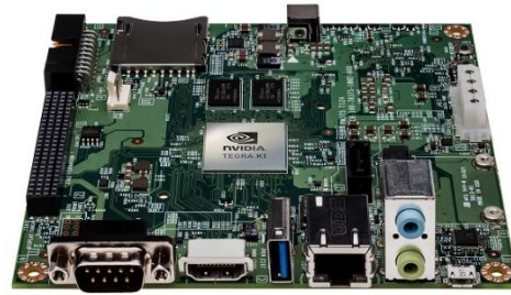
Jetson TK1 Development board vista superior
